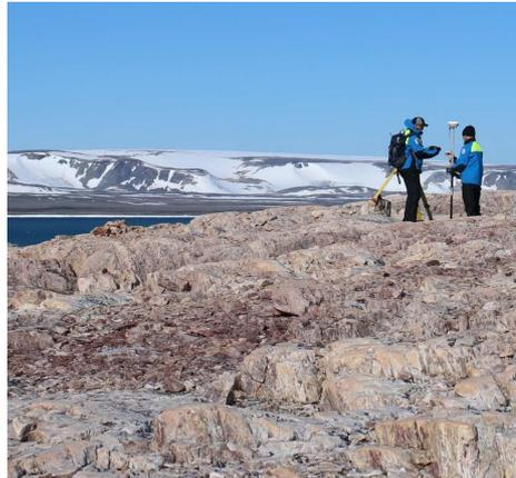
In photo, single station RTK is used by KTH personnel in the Arctic, Spitsbergen, where the infrastructure is very sparse
