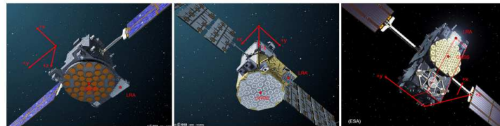
Fig. 1 Spacecraft reference system and sensor location for the GIOVE-A (left), GIOVE-B (center) and Galileo-IOV (right) satellites (images: ESA). Note that the Sun incidence direction in the artist's drawings of GIOVE-A and GIOVE-B does not comply with the true attitude control of the two spacecraft, which always keeps the Sun in the -x-hemisphere.
